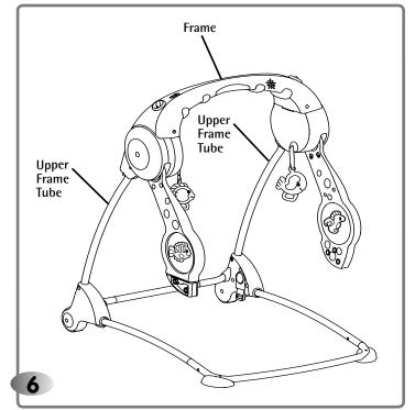
• Check to be sure the upper frame tubes are secure in the frame. If you can remove the upper frame tubes from the frame, you have not properly inserted the tubes into the frame. Repeat Assembly step 5.
